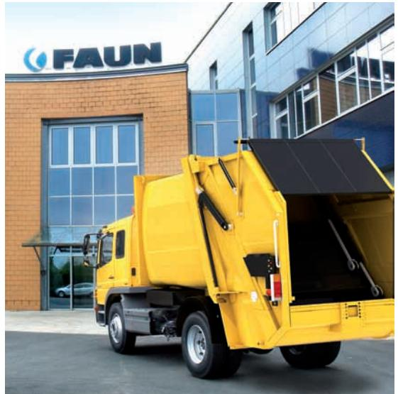
FAUN VARIOPRESS 2.30 m wide on twin-axle chassis
